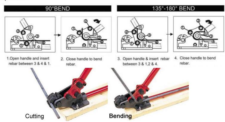
**Note:** This tool is for cutting & bending rebar only. Maximum capacity is #5 (5/8") Grade 60 rebar. Top cutting slot is for #4 (1/2") & #5 (5/8") lower slot is for #3 (3/8") rebar. Cutting or bending any other material is considered misuse. The Equipment Protection Plan does not cover damages caused by misuse.
