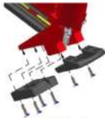
FIGURE 4 Tongue Nailing 9/16\" Flooring Shoe P/N 50125 Shoe Base P/N 50184 (Black) Shoe Pad P/N 50181 (Black)
